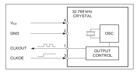
PIN CONNECTIONS TOP VIEW:
